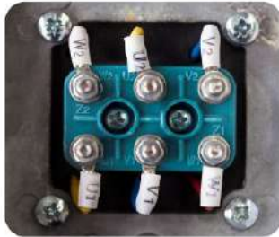
MOTORS WITH 6 TERMINALS DUAL POLARITY 2 WINDINGS
